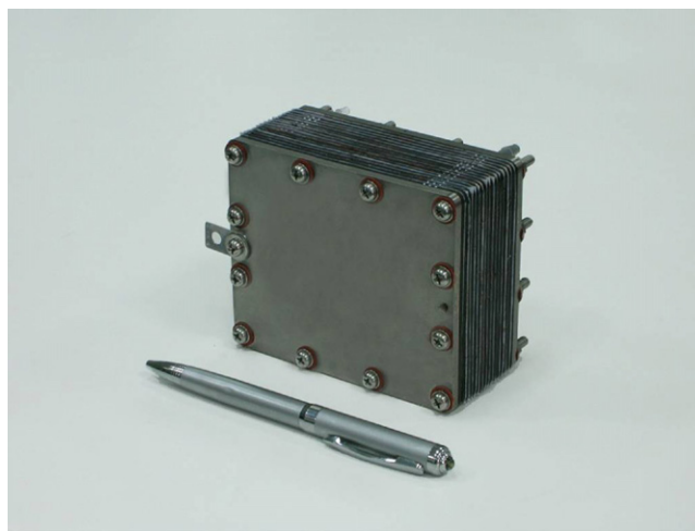
Fig. 1. An experimental 16-cell bipolar plate stack.
