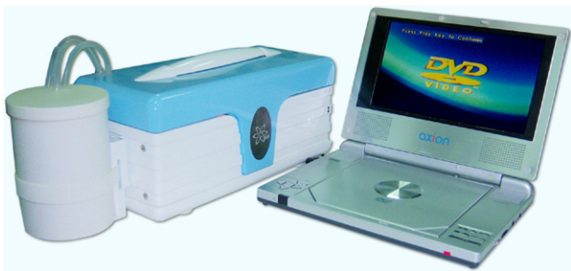
Fig. 13. Demonstration of a DVD player powered by a 40 W DMFC system.
